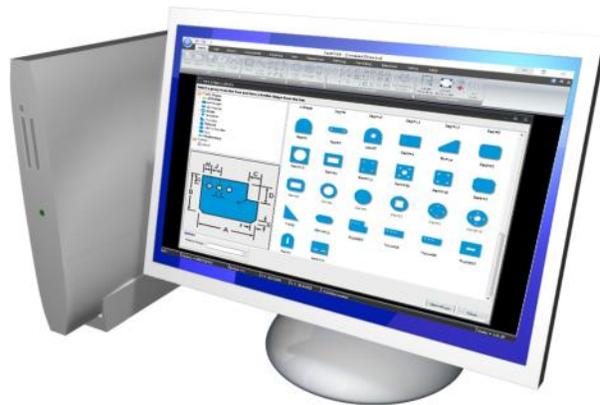
Simple drafting, editing and verification of geometry to create **precise 2D and bevel parts** that can be used in NC quotation, nesting & production.
